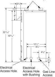
Figure 2 - Firebox Side View
